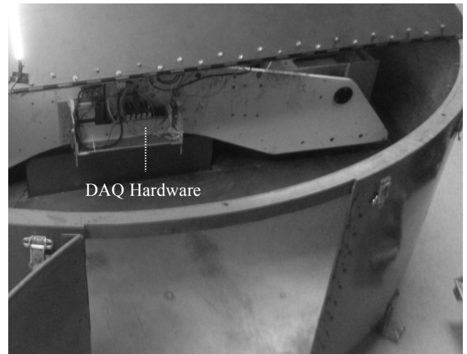
Figure 3. NI instruments location in the USC centrifuge.
